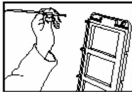
6. Drill one hole through the wall for the passage of the low-voltage wiring in the location as shown on the template.
